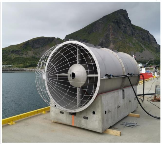
Nova Sea provides an "oxygen feast" for its farmed salmon via new seawater pump technology
